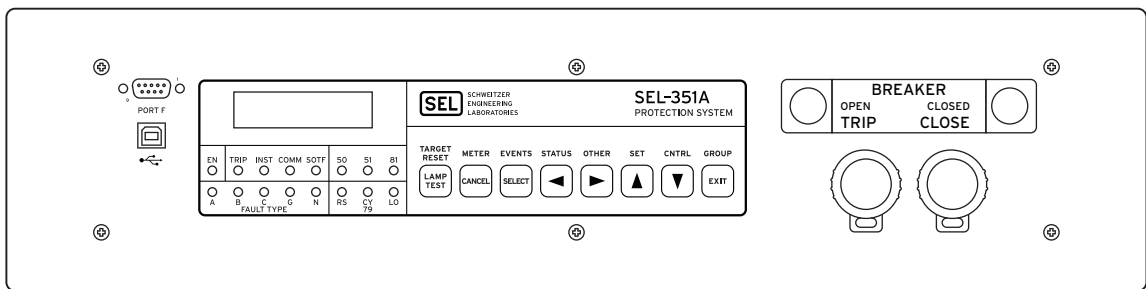
Panel or Projection Mount With USB Port and SafeLock Trip/Close Pushbuttons
